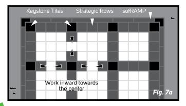
The final tile located in the middle of the strategic row is the compression tile and must be compressed into place last.
